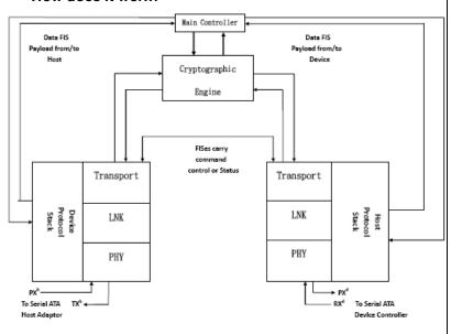
The X-Wall MX+, an SATA-to-SATA cryptographic ASIC, sits right in between host SATA adapter and the device SATA controller, encrypting entire SATA drive with wire speed performance while providing 256-bit AES hardware strength in ECB, CBC or XTS mode of operation.
